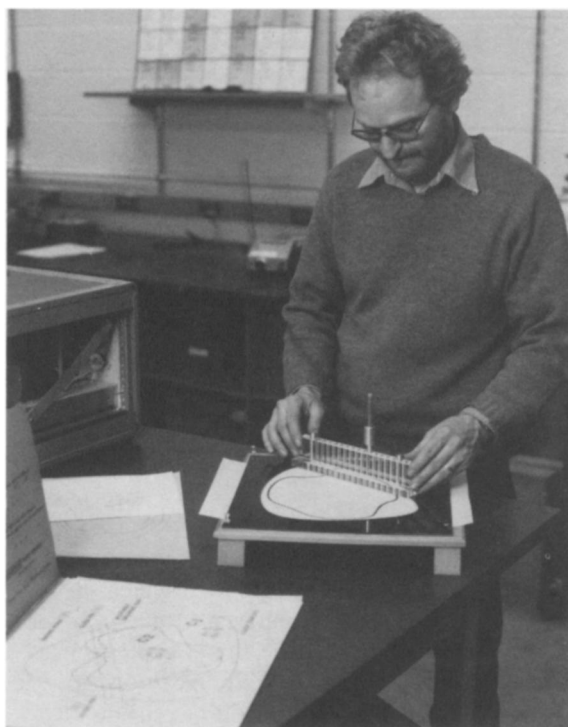
Dan M. Pomeroy operates the Holditch drawing-bar. The guide template is the same as in FIGURE 1; curve c_1 is being drawn.
